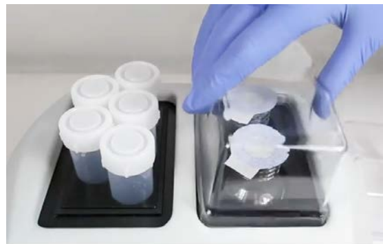
CH-3 thermostat with block B5-29 (left) and block B2-50 (right)
