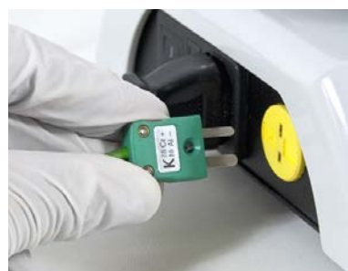
Connection of the external probe, rear side MSH-300i
