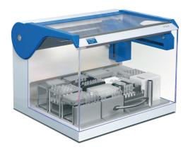
PIRO pipetting robot provides extreme flexibility in combination with small space for various liquid handling tasks. Whether simple fluid transfer or complex PCR run, with the easy to use software your application is ready within minutes.
