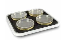
Flat Platform with non-slip silicon mat for Petri dishes, culture flasks and agglutination. Working area: 230 x 230 mm Order No. 105.1218
