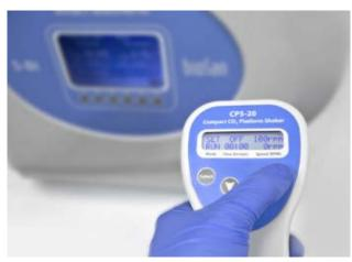
The remote control minimises disturbances to the incubator environment and the experiment in progress. The unit controller is designed for operation in cold rooms, incubators and closed laboratory rooms at ambient temperature from +4°C to +40°C in a non-condensing atmosphere and relative humidity up to 80% for temperatures for temperatures up to 31°C decreasing linearly to 50% relative humidity at 40°C.
