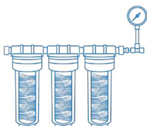
External polyphosphate/carbon filter
