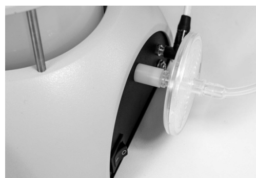
Rear side with ON/OFF switch and hydrophobic microbiological filter
